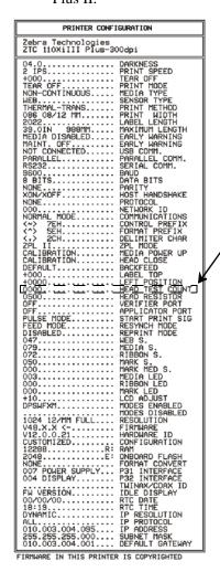
If the Head Test Option is installed, HEAD TEST COUNT will be listed.
